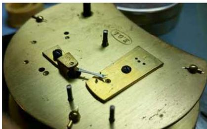
The balance has its own lower jewel setting in a small separate plate screwed onto the back plate. The balance bridge, with hairspring and regulator, is screwed into that. There is no adjustment.
